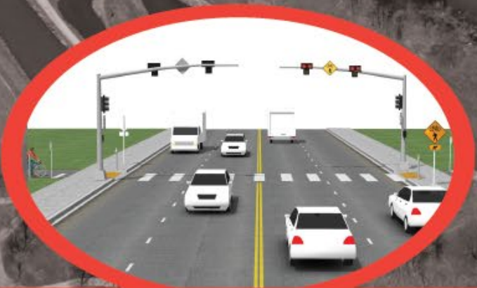
HYBRID BEACON CROSSING AT INTERSECTION WITH ADVANCED WARNING SIGNAGE
